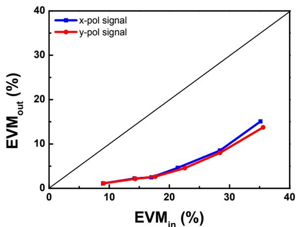
Fig. 8. EVM of the PDM DPSK signals before and after PR.
