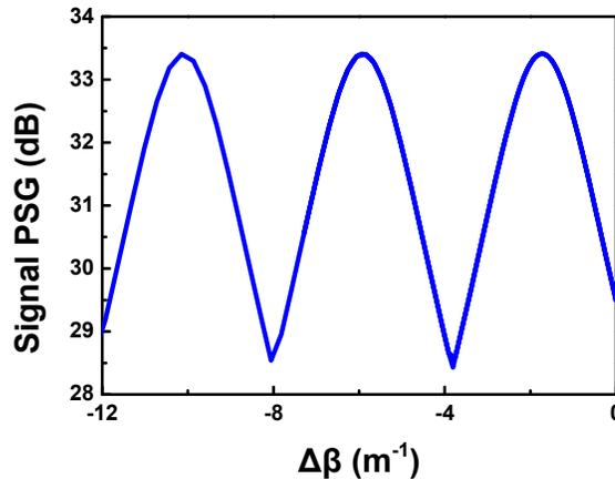
Fig. 4. Calculated signal phase sensitive gain (PSG) as a function of the linear phase matching factor,  $\Delta\beta$ .
