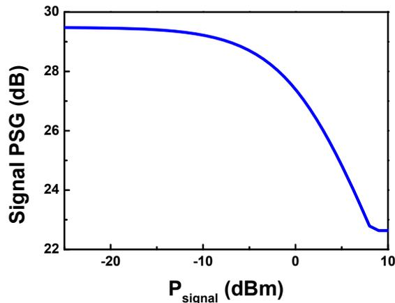
Fig. 5. Calculated signal phase sensitive gain (PSG) as a function of the signal power,  $P_{signal}$ .
