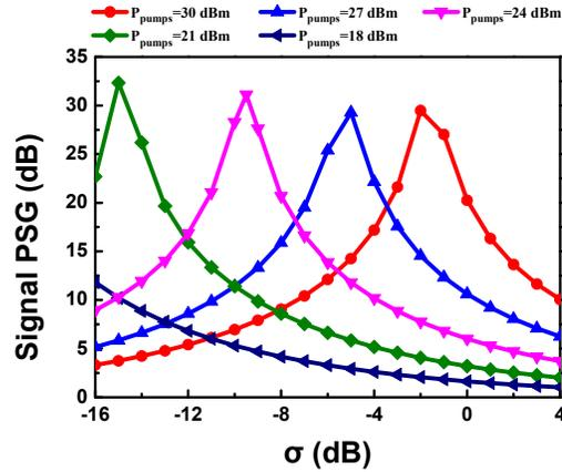
Fig. 3. Calculated signal phase sensitive gain (PSG) as a function of the input signal-to-idler ratio  $\sigma$  for different total pump power,  $P_{pumps}$ , i.e.  $P_{pumps} = 18, 21, 24, 27$  and  $30$  dBm.
