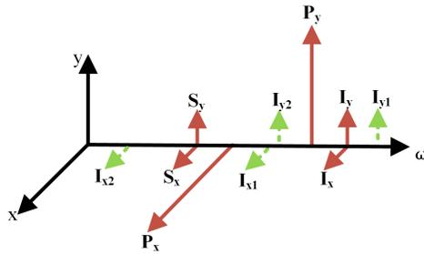
Fig. 1. Polarization and frequency diagram for vector dual-pump nondegenerate PSA processes for PDM PR.  $P$ : pump;  $S$ : signal;  $I$ : idler.  $x$  and  $y$  denote two orthogonal polarization states. Red solid line: launched wave; green dash line: generated line.
