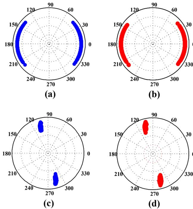
Fig. 7. Simulated constellation of PDM DPSK signals: (a) x-pol signal without PSA; (b) y-pol signal without PSA; (c) regenerated x-pol signal; (d) regenerated y-pol signal.
