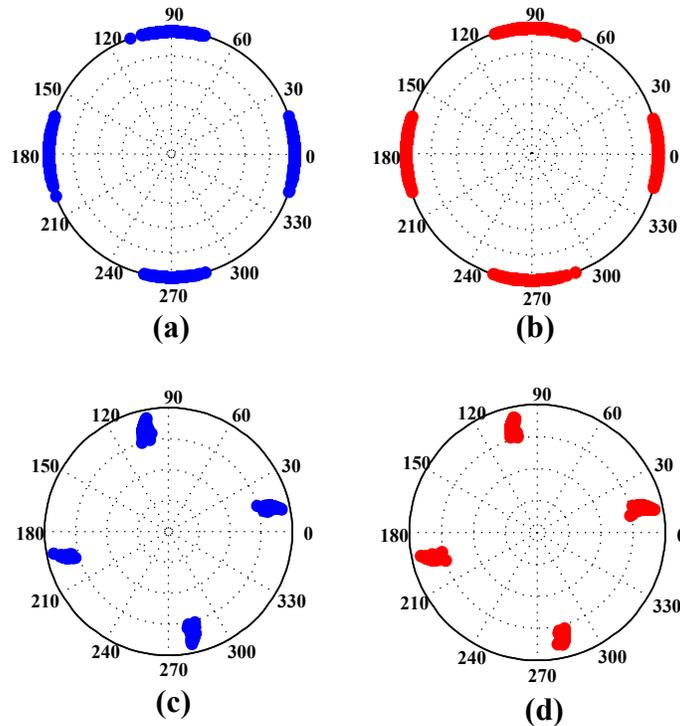
Fig. 9. Simulated constellation of PDM QPSK signals: (a) x-pol signal without PSA; (b) y-pol signal without PSA; (c) regenerated x-pol signal; (d) regenerated y-pol signal.
